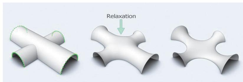
◀ Figure 7. Surface minimization (left to right): rest length reduction
